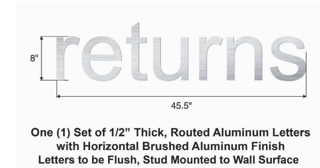
One (1) Set of 1/2" Thick, Routed Aluminum Letters with Horizontal Brushed Aluminum Finish Letters to be Flush, Stud Mounted to Wall Surface 60493 City of Louisville
