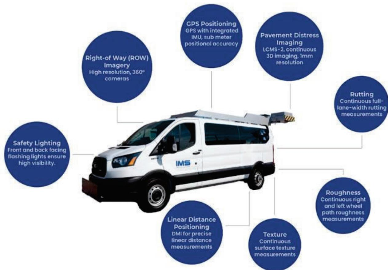
*IMS Road Surface Tester (RST) equipped with Laser Crack Measurement System (LCMS-2)
