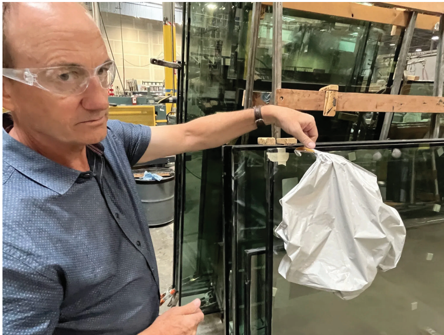
Craig Maierhofer with proprietary lung or balloon that permits expansion during transit. Ken Amundson/BizWest
