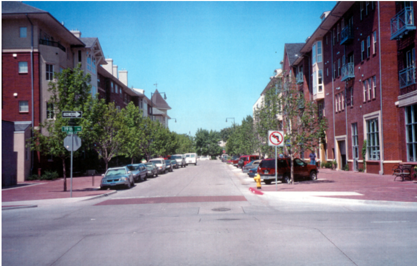
Multifamily streetscape on a local roadway in Denver The fifth story living space is accommodated within the roofs of buildings. Sidewalk bumpouts, differentiated pedestrian crossings, and on-street parking help to calm traffic.
