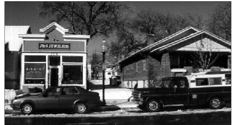
Develop the ground floor level of all projects to be at a pedestrian scale. Porches and large areas of glass are both appropriate treatments.
