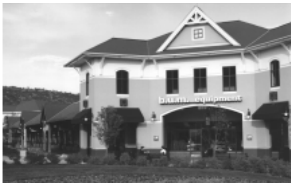
4.3 B & C USE A VARIATION IN FACADE ELEMENTS TO REDUCE PERCEIVED SCALE.
