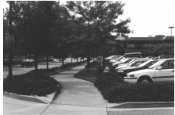
3.1 B SEPARATE PEDESTRIAN AND VEHICULAR MOVEMENTS WITH LANDSCAPING, BARRIERS, OR OTHER APPROPRIATE DESIGN SOLUTIONS.
