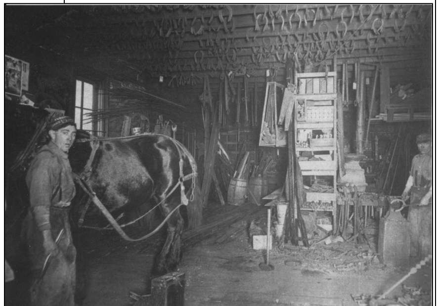
In this photo of the interior of Bob Stretz's blacksmith shop, he is standing on the right and can be seen working on shaping a horseshoe. The man on the left is unidentified. Note the horseshoes hanging from the ceiling.
