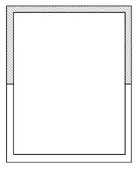
(c) Any exterior wall facing a public street, but not an act or process which removes an exterior wall facing an alley (see diagram). The shaded area illustrates the maximum amount that may be removed without constituting demolition as defined by this provision.
