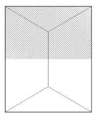
(b) Fifty percent or more of the exterior walls of a building as measured contiguously around the building (see diagram). The shaded area illustrates the maximum amount that may be removed without constituting demolition as defined by this provision.
